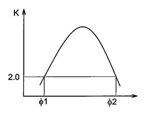
Viewing Angle Contrast ratio K vs viewing angle  $\phi$
