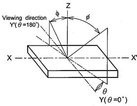
Note 2: Definition of viewing angle  $\phi 1 < 0^{\circ} < \phi 2$
