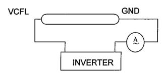
Note 7: We recommend to equip protection circuit (to stop output) which works under abnormal operation to the inverter for CFL.
